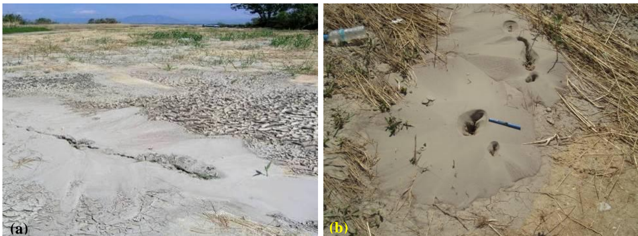
Figure 3. Cone ejecta at SITE-I, in the coastal zone of K. Achaia following the 8-6-2008 earthquake: (a) gray silty sand (SM), (b) brown sand (SP).
