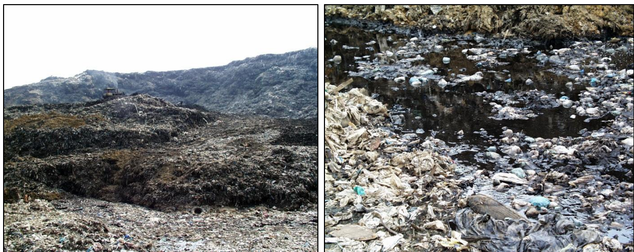
Figure 8. Composition of waste mass in slide area with no soil cover (photos by S.M. Merry).
